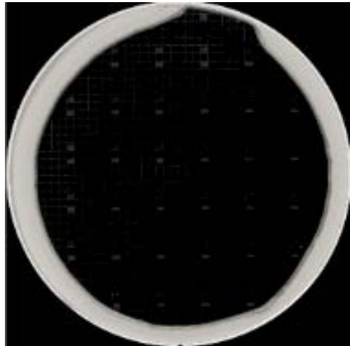
Pair 3: Si/Si, Edge de-bonding after final anneal
